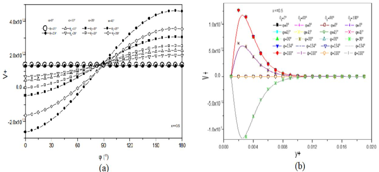
**Figure 9.** Evolutions of the dimensionless normal component  $V^+$  as a function of the dimensionless azimuthal and normal coordinates
