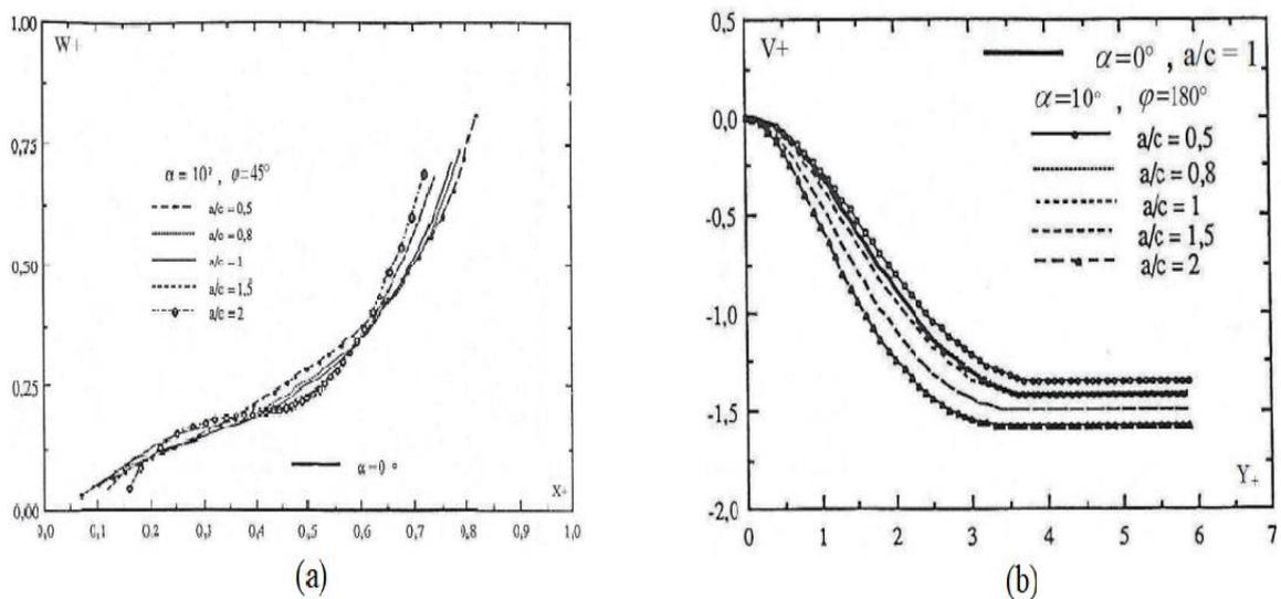
**Figure 7.** Variations of the dimensionless normal component  $V_+$  as a function of the dimensionless meridian and normal coordinates, for several values of  $a/c$
