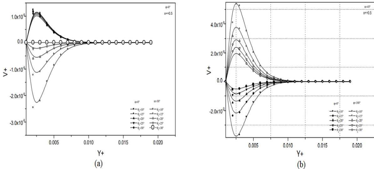
**Figure 6.** Variations of the dimensionless normal component  $V_+$  against the dimensionless normal coordinate  $y_+$ , for several values of  $\theta_0$ ,  $\alpha$  and  $x_+=0.5$
