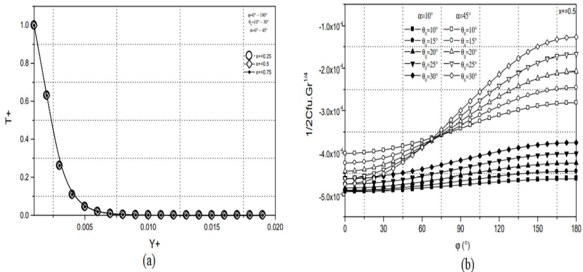
**Figure 8.** Evolutions of the dimensionless temperature  $T^+$  and the meridian or tangential friction coefficient
