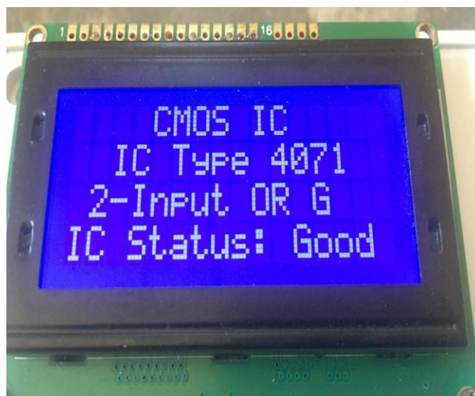
Fig 10 One of the results of testing 4071 CMOS IC with the Improved IC Multi-Tester.
