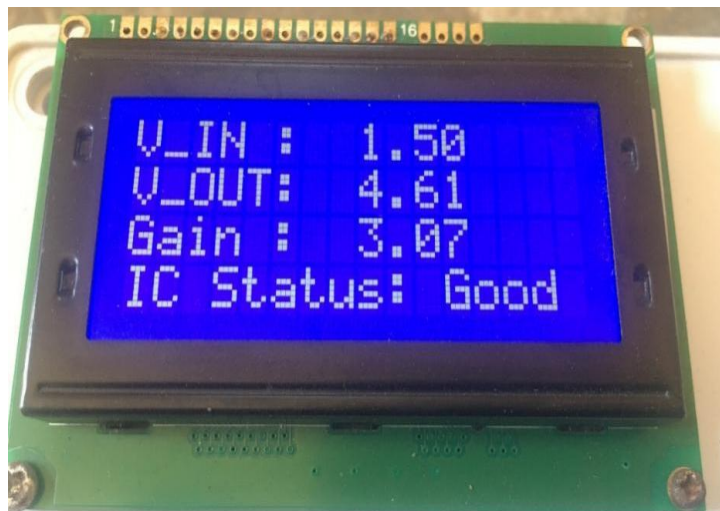
Fig 9. One of the results of Testing Op-Amp IC with the Improved IC Multi-Tester.
