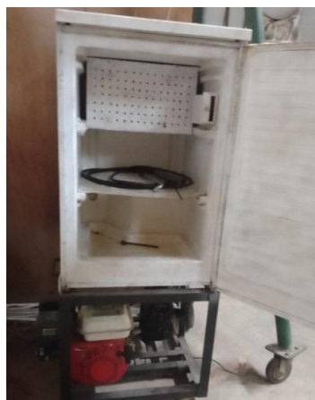
Figure 3: Assemblage of Gasoline-driven Refrigeration System
