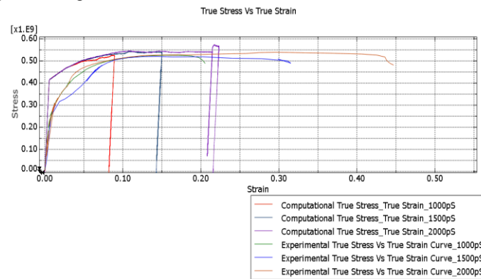
Fig. 6. Computational and experimental true stress vs true strain at 1000, 1500, 2000s -1
