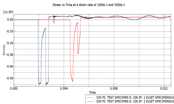
Fig. 8. Stress vs time at a strain rate of 1000s -1 and 3500s -1
