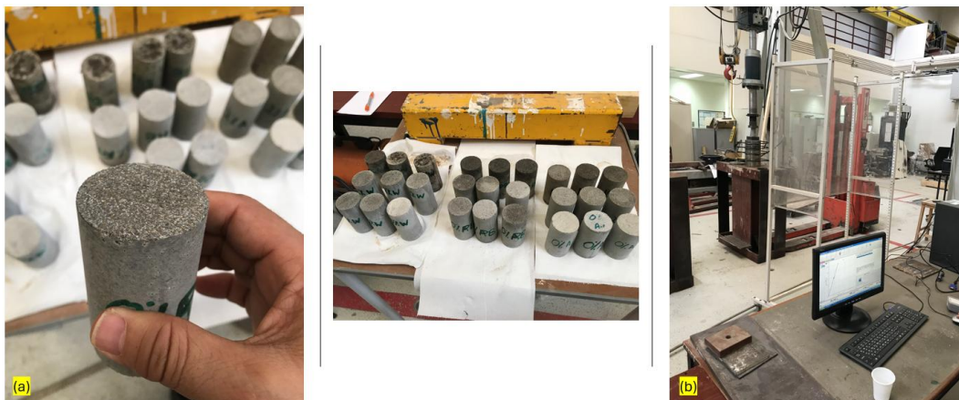
Figure 4 Compressive strength machine
