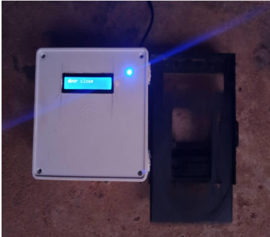
Figure 3.10: When the door is closing after waiting for 4second
