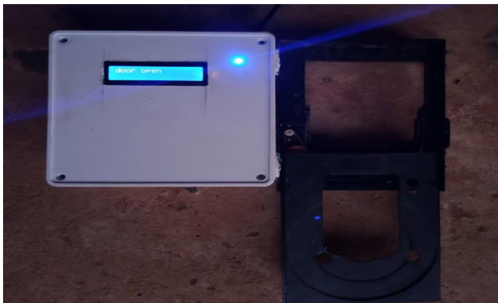
Figure 3.9: When password is entered in the terminal and the door is opening
