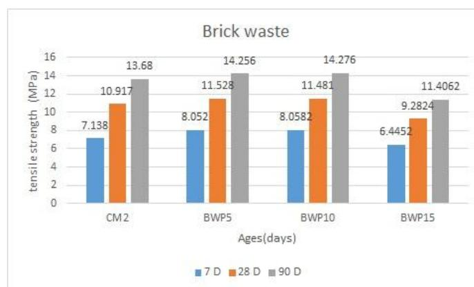
Figure 8 The effect of brick waste on tensile strength.
