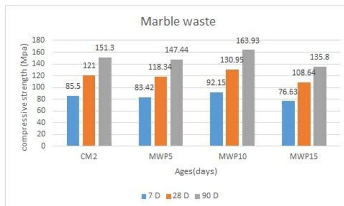
Figure 5 The impact of marble waste on compressive strength
