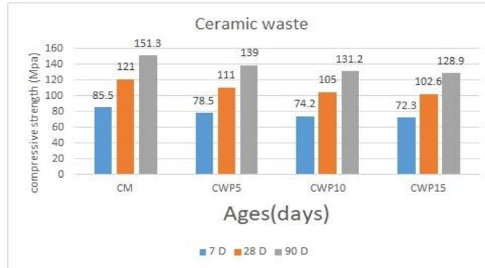
Figure 3 The ceramic impact on compressive strength
