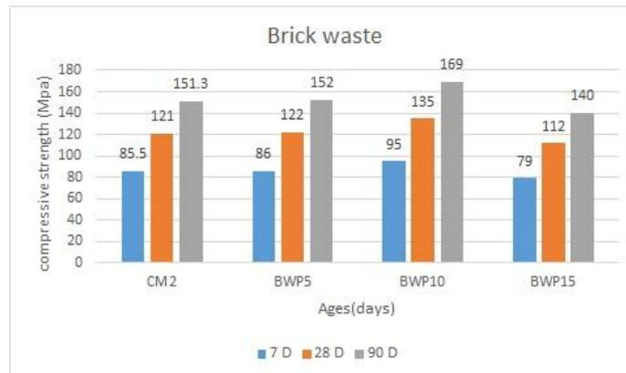
Figure 4 The impact of Brick waste on compressive strength
