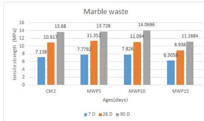
Figure 9 The impact of marble waste on tensile strength
