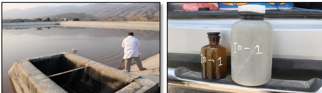
Fig. 4.1 How to take a sample from the basin
