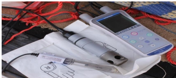
Fig. 4.6 The field device (HORIBA – PH/DO METER D-55)
