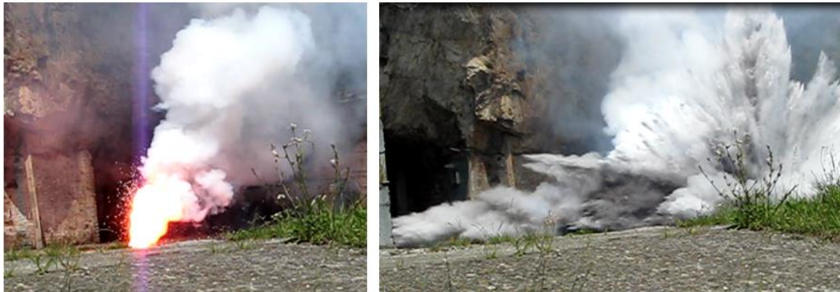
Figure 5 Practical test of the water spout in extinguishing a flame caused by the use of PS-25
