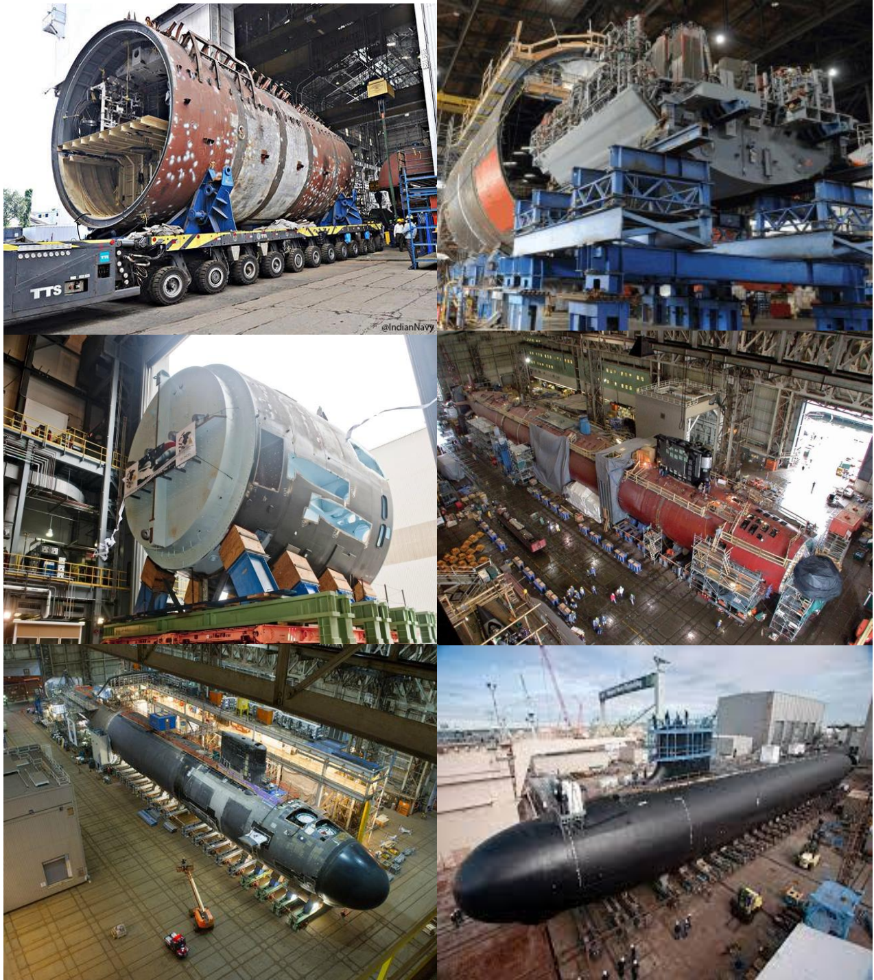
Figure 13: Modular Construction of Submarine (Virginia-class Nuclear Power submarine of the US Navy) 37
