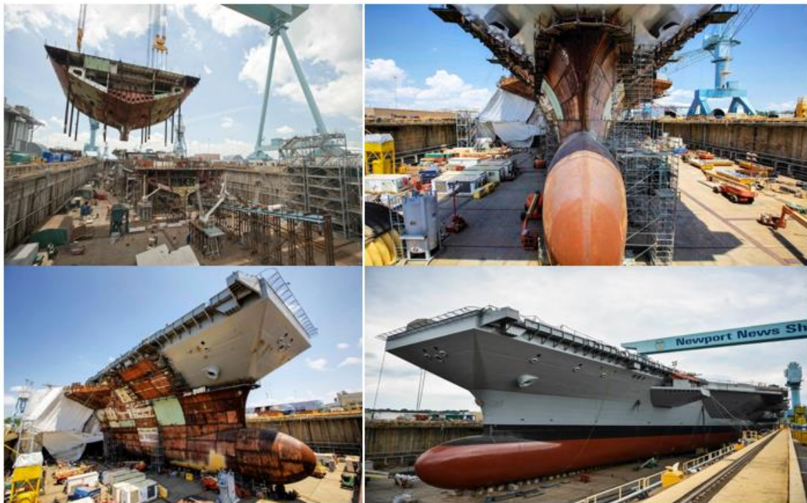
Figure 14: Modular construction of modern aircraft (Aircraft Carrier Gerald R Ford of the US Navy) 38
