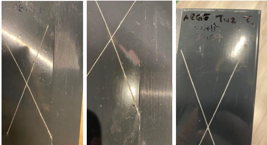
Fig. 3 Dyed AA1050, AA6063 and AA6082 Aluminium Profiles (Acidic Acid Test)
