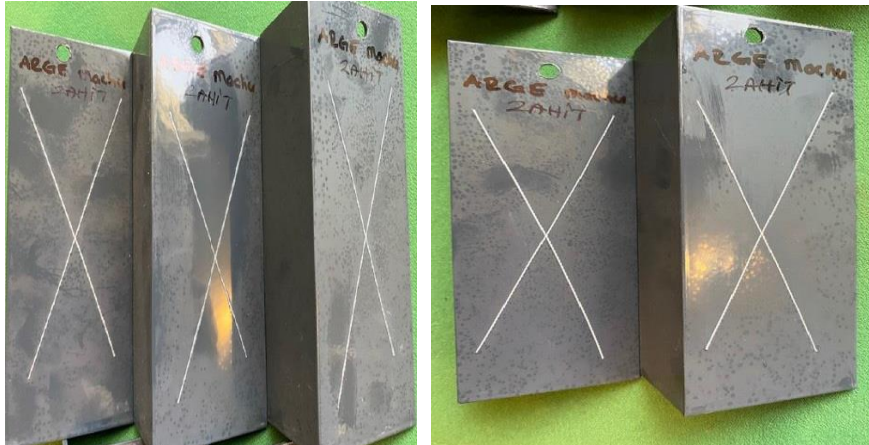
Fig. 2 Dyed AA1050, AA6063 and AA6082 Aluminium Profiles (Machu Test)
