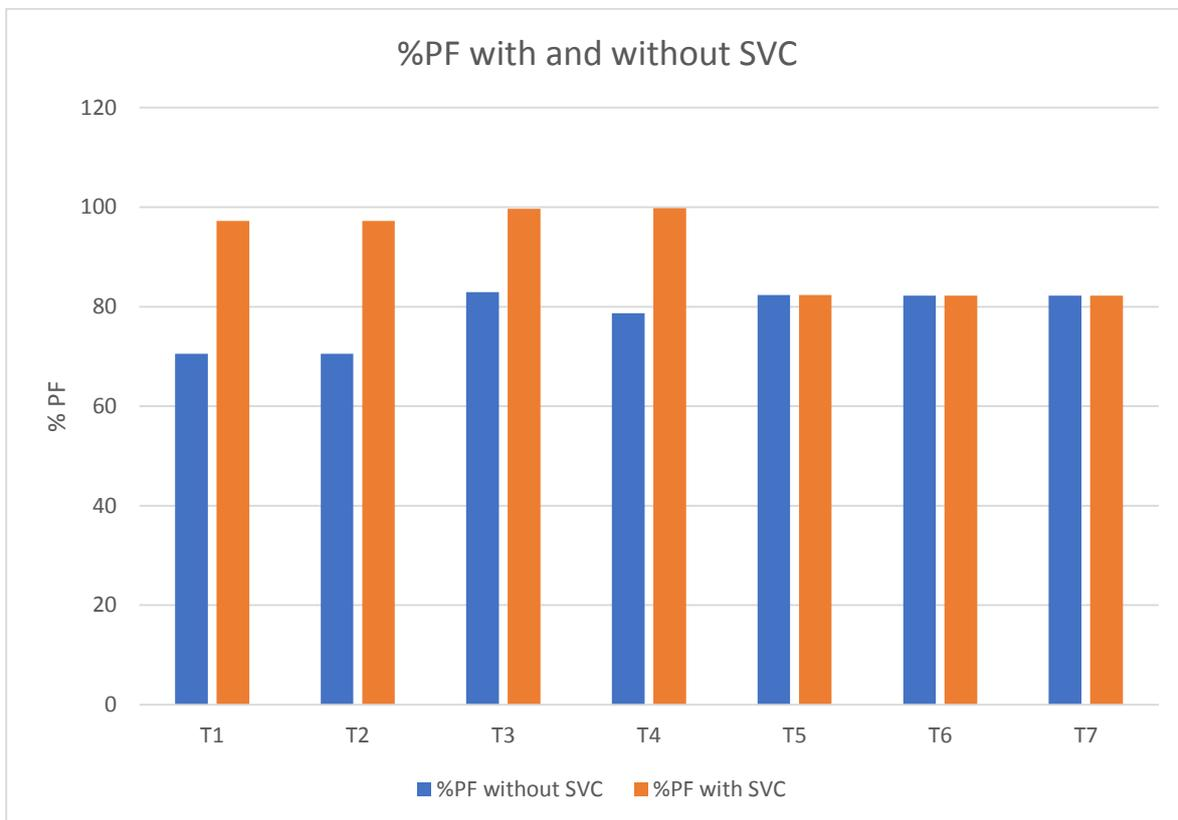
Fig. 9: % Power factor with and without SVC
