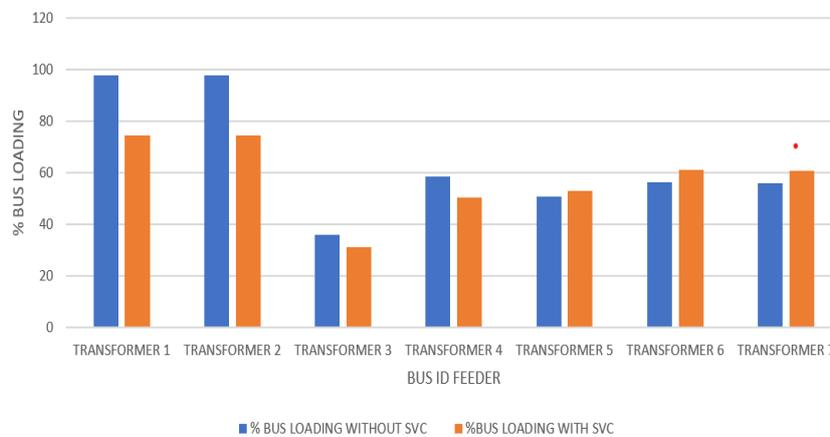
Fig 5: Chart showing % Bus loading with and without SVC
