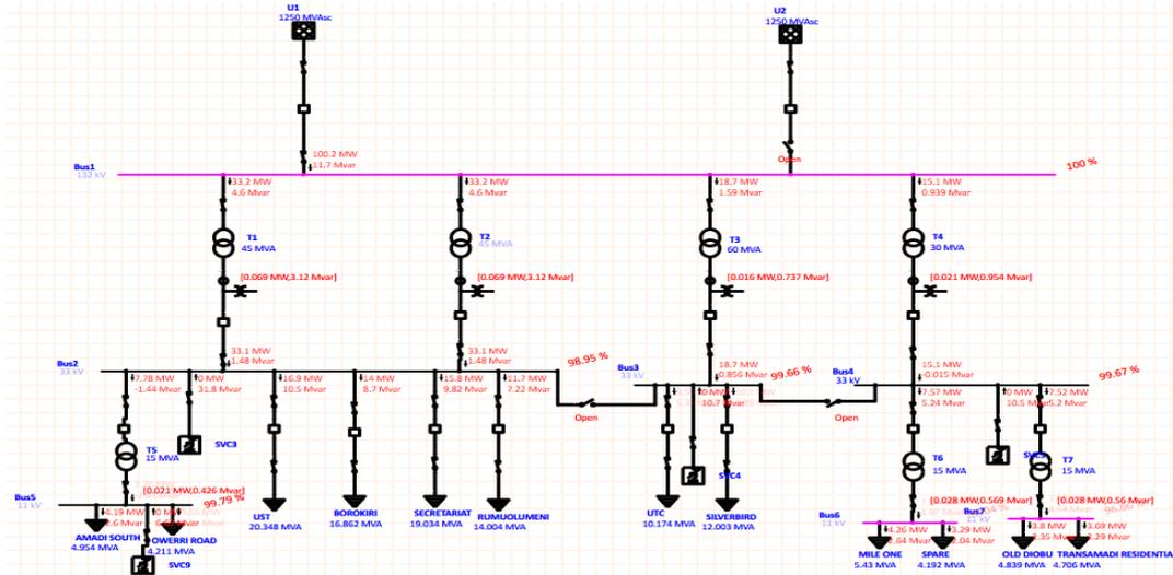
Fig. 4: LFA of the base-case network with SVC compensation
