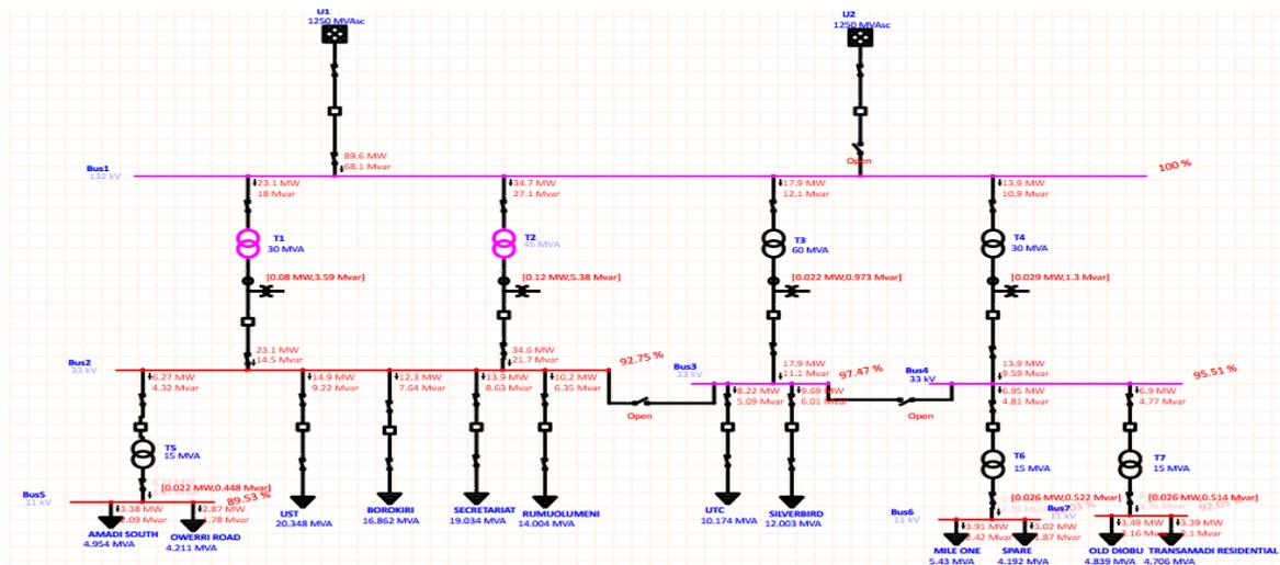
Fig. 3: LFA of the base-case network without SVC
