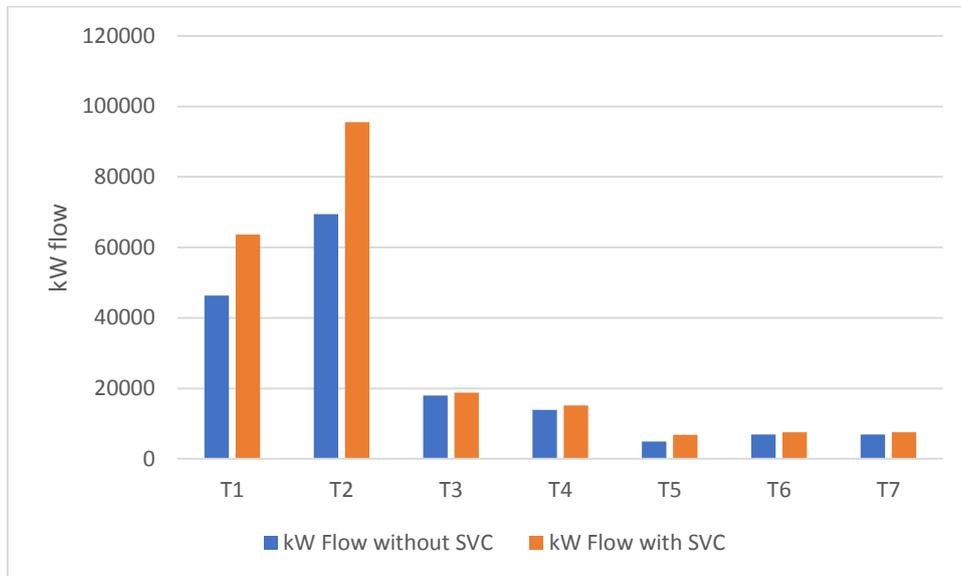
Fig. 7: kW flow with and without SVC
