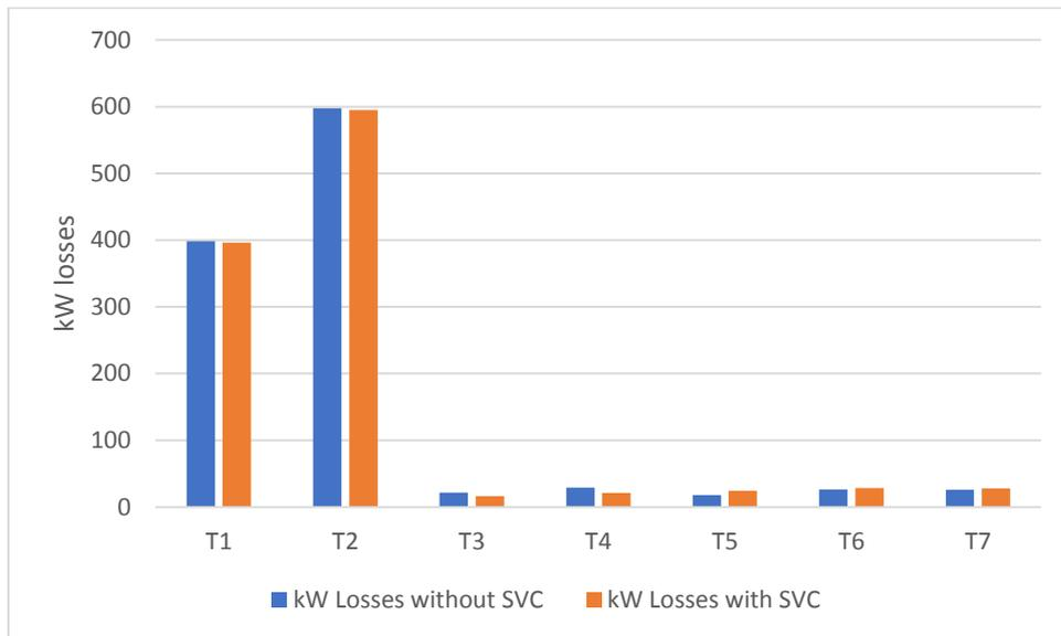
Fig. 8: kW losses with and without SVC
