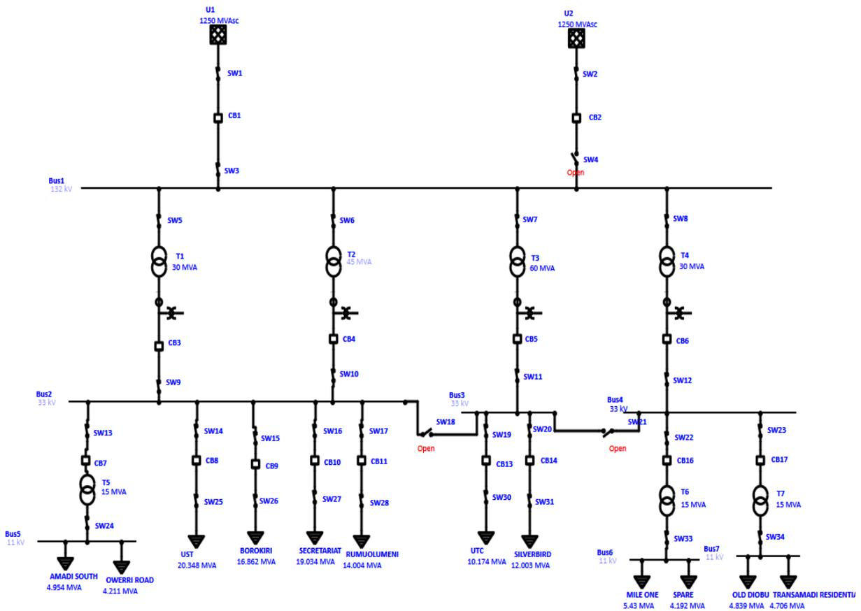
Fig. 2: The Single Line Diagram of Port Harcourt Town 132/33kV Substation
