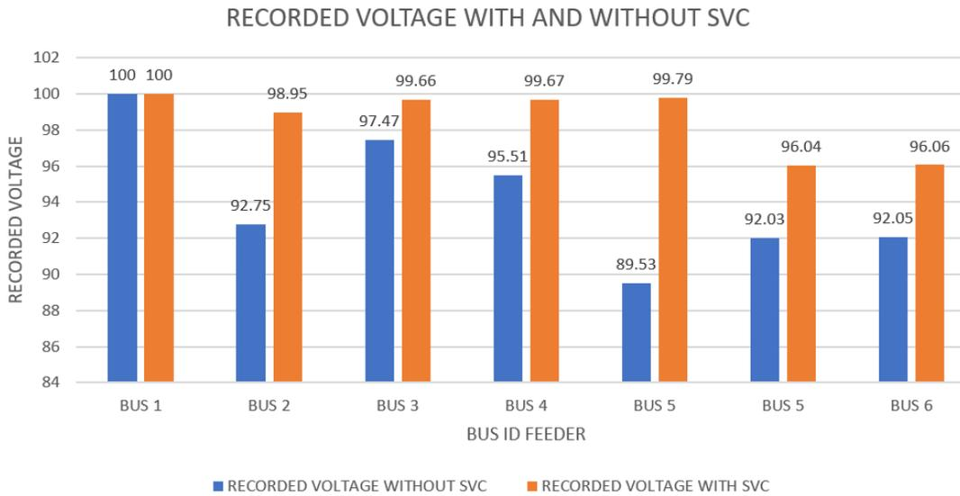
Fig 6: Recorded voltage with and without SVC
