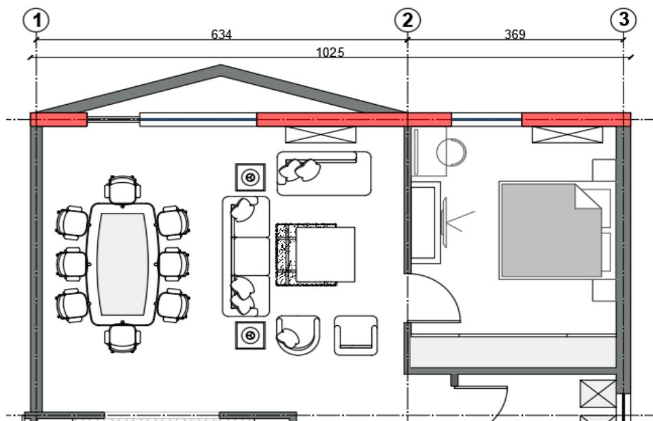
**Fig. 13 Floor plan of the apartment (Building A).** The measurements were performed on the perimeter wall showed in red. Source: Authors
