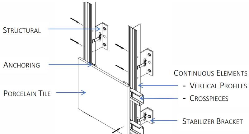
**Fig.1 Hidden anchoring system. Source [9]**
