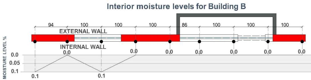
**Fig.20 Interior moisture graph for Building B, Source: Authors**
