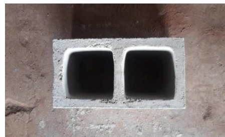
Fig. 3.2: A 2-Cell molded sandcrete hollow block
