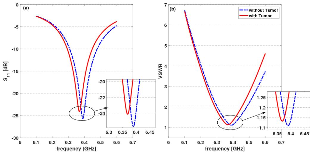
Figure 13. (a) The return loss and (b) the VSWR for the design P3 with and without tumor.
