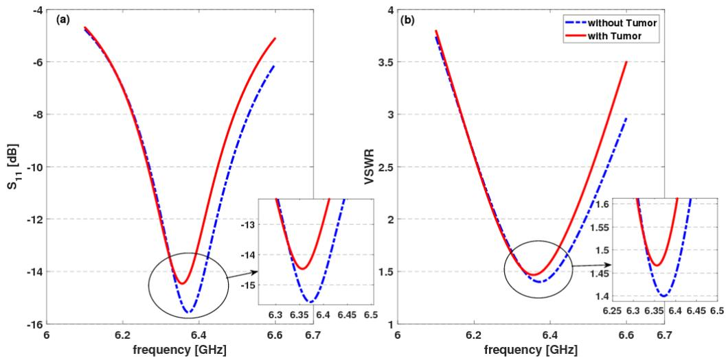
Figure 12. (a) The return loss and (b) the VSWR for the design P2 with and without tumor.
