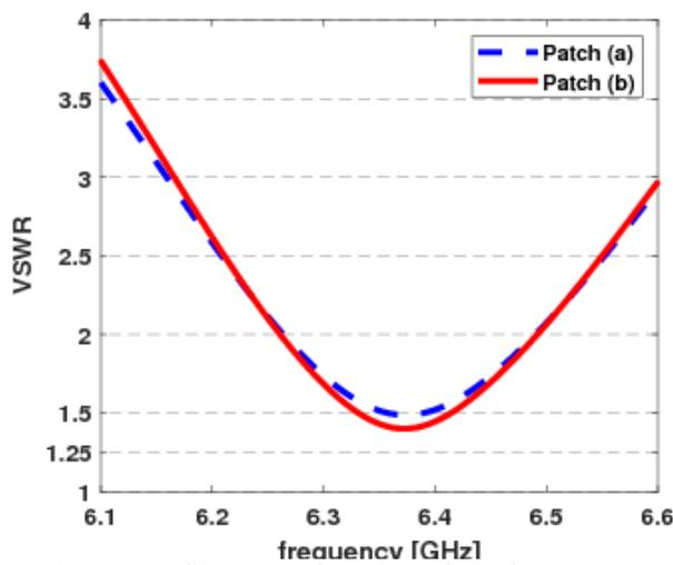
Figure 6. VSWR as a function of the frequency
