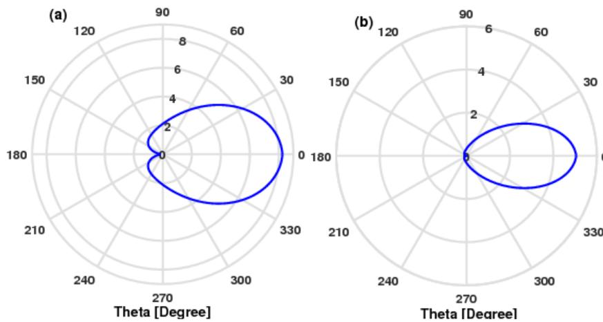
Figure 10. (a) Field radiation pattern and (b) directivity radiation pattern
