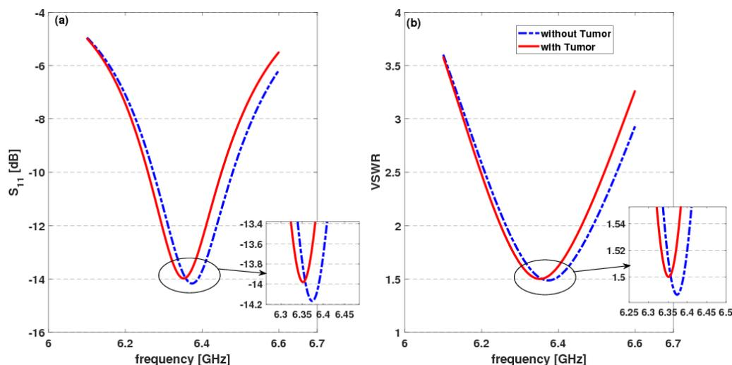
Figure 11. (a) The return loss and (b) the VSWR for the design P1 with and without tumor.
