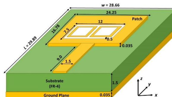
Figure 2. Illustration of patch antenna dimensions.
