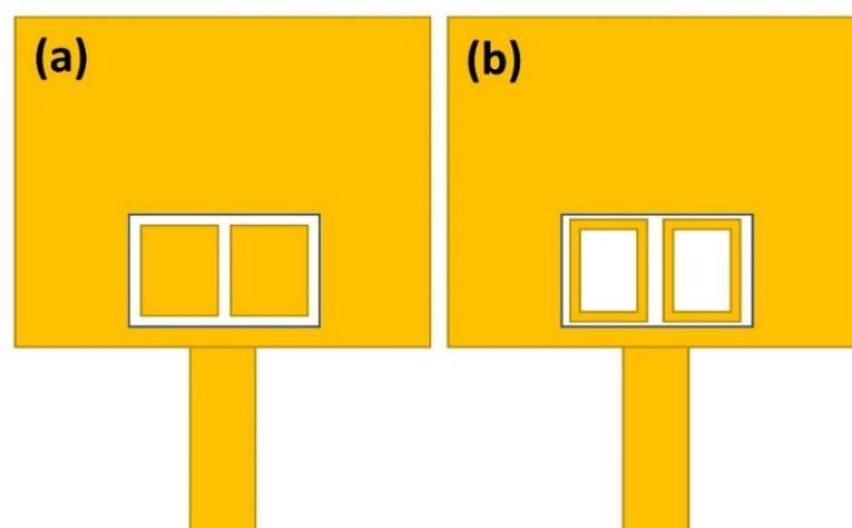
Figure 4. (a) Initial model of the patch antenna (P1), and (b) modified model (P2).
