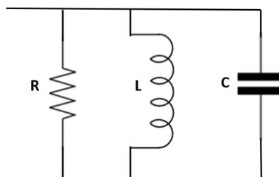
Figure 1. Equivalent circuit of the rectangular patch antenna.
