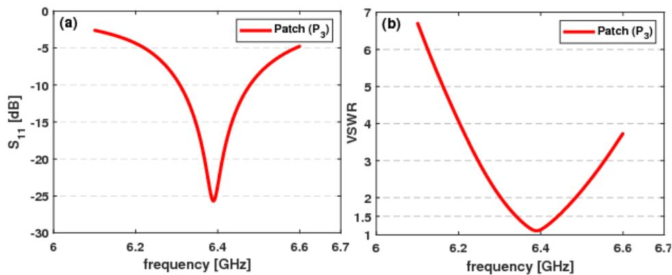
Figure 9. (a)  $S_{11}$  parameter as a function of the frequency and (b) variation of the VSWR with frequency.
