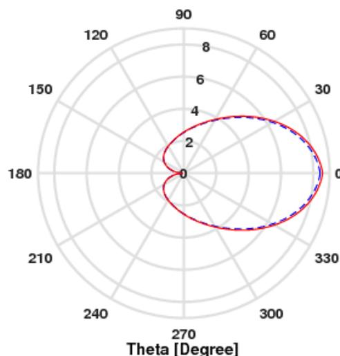
Figure 7. Comparison between the field radiation pattern of P1 (blue dotted line) and radiation pattern of P2 (red solid line) at the resonance frequency.
