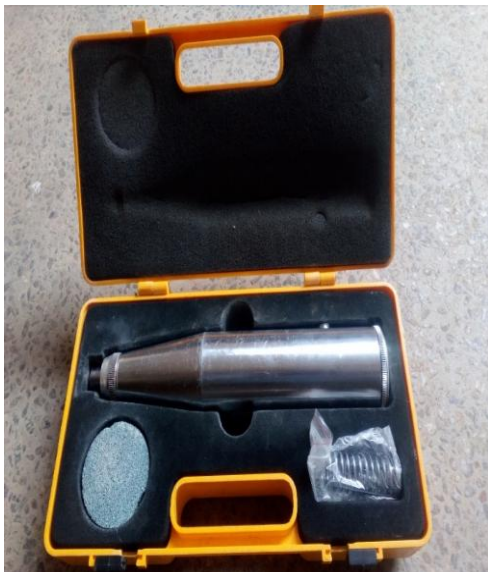
Fig. 3: Schmidt Rebound Hammer Fig. 4: Pundit Lab Equipment
