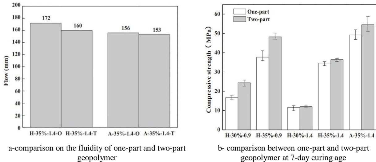
Note; T: two-part geopolymer, H: hydrous sodium silicate (Na<sub>2</sub>SiO<sub>3</sub>), O: one-part geopolymer and A: anhydrous sodium silicate (Na<sub>2</sub>SiO<sub>3</sub>).
