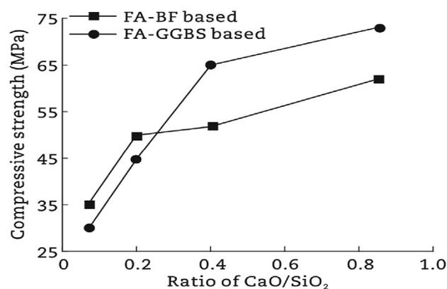
Fig. 7: The variation of compressive strength at room temperature, BF (bazalt fiber), [105].
