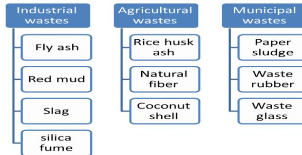
Fig. 3. Solid wastes that used in geopolymers concrete [30].
