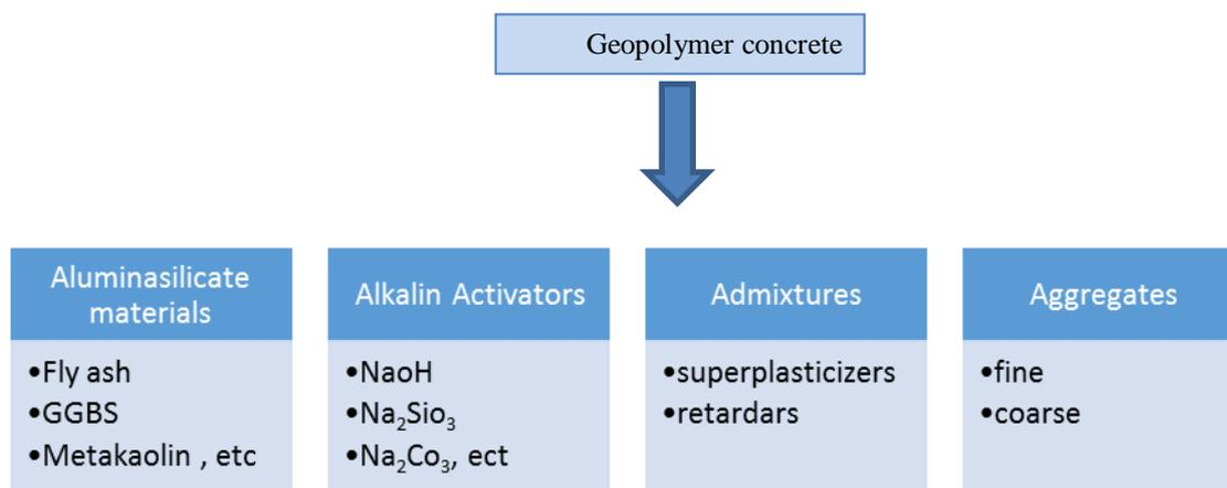
Fig.2. Constituents of geopolymer concrete [28],[29].
