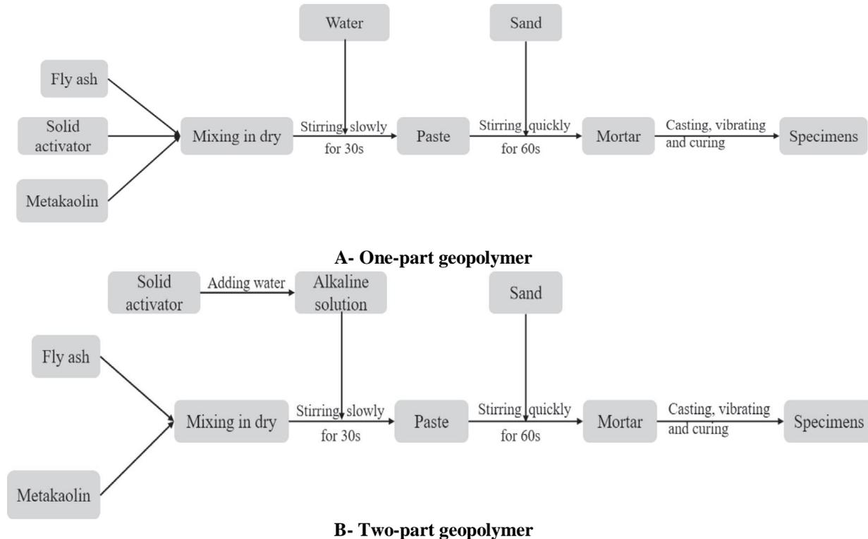
**Fig. 4. Preparation methods of geopolymers concrete [43].**
