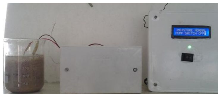
Fig.3.6 showing soil moisture status and pump status displayed on a LCD screen.
