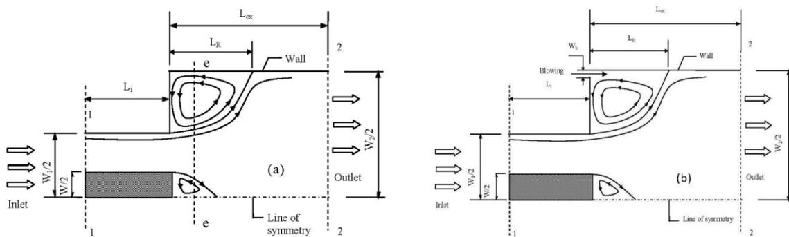
Fig. 1. Schematic diagram of the computational domain (a) Model-1 (b) Model-2
