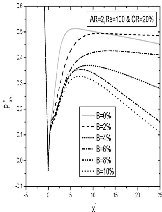
Fig. 2 Effect of blowing on average static pressure distribution
