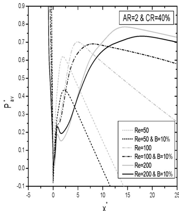
Fig. 4 Effect of Reynolds number on average static pressure distribution
