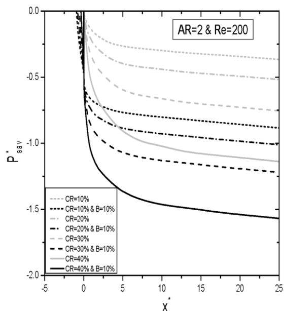
Fig. 7 Effect of central restriction on average stagnation pressure distribution
