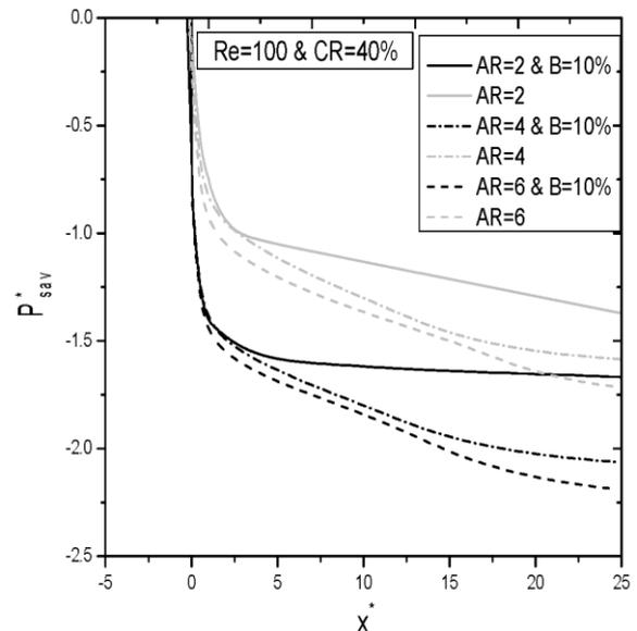
Fig. 9 Effect of aspect ratio on average stagnation pressure distribution
