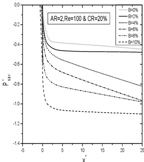
Fig. 6 Effect of blowing on average stagnation pressure distribution
