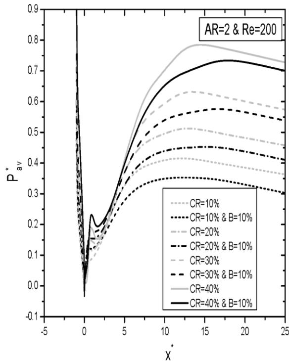
Fig. 3 Effect of central restriction on average static pressure distribution
