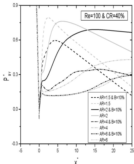
Fig. 5 Effect of aspect ratio on average static pressure distribution
