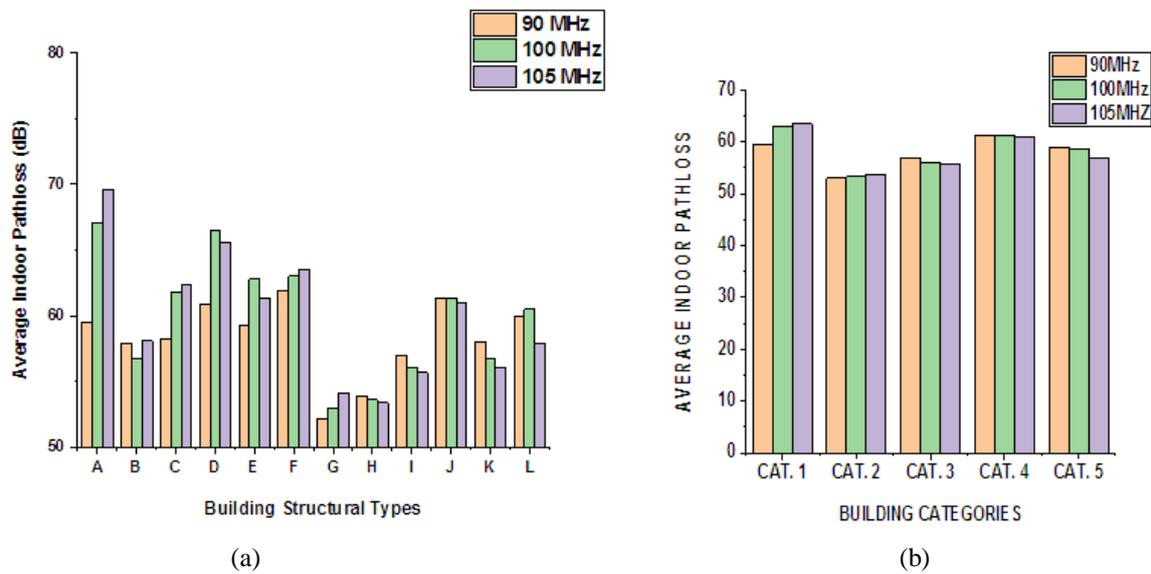
Figure 3: (a) Average Indoor Path loss of the selected buildings structures at (90, 100 and 105) MHz (b) Average Indoor Path loss against building categories at (90, 100 and 105) MHz
