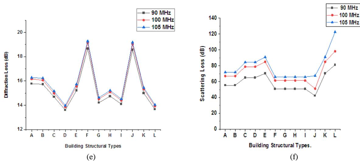
(e) Estimated diffraction loss against building materials and structural types (f) Estimated scattering loss against building materials and structural types
