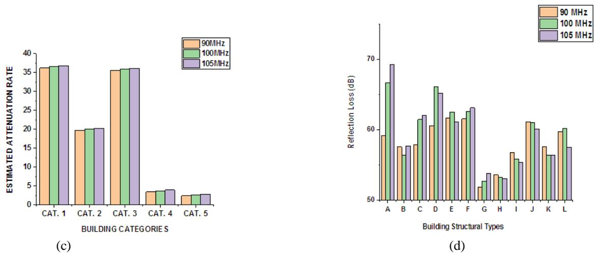
(c) Estimated Attenuation rate (dB) against building categories (d) Estimated reflection loss against building materials and structural types
