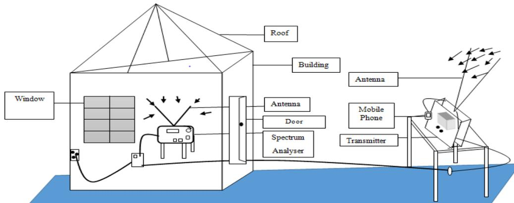
Figure 1: Building geometry and instrumentation configuration
