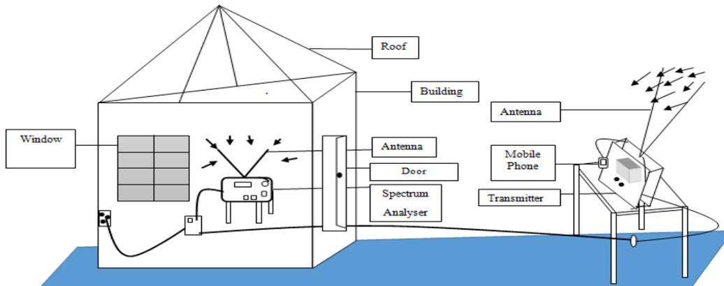
Figure 1: Building geometry and instrumentation configuration
