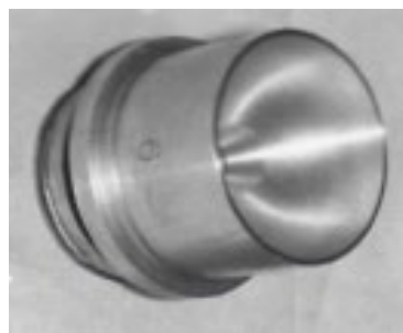
Fig. 6 Experimental model of a shortened nozzle with a total length of 40 mm
