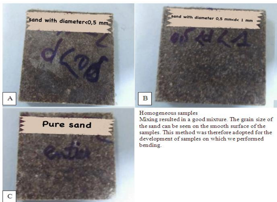
Fig. 6. Homogeneous samples with 3 different types of mixture , pure sand , sand with d < 0,5 mm and 0,5 < d < 1 mm
