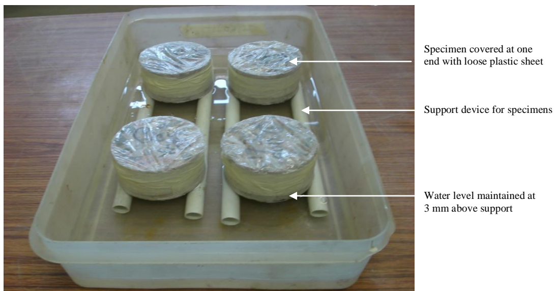
Fig. 1: Sorptivity test specimens
