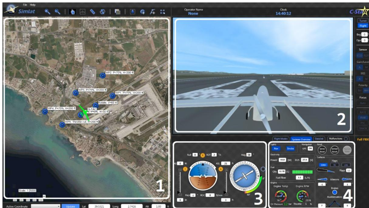
**Fig. 4. Pilot station screen divided into four zones of interest**
