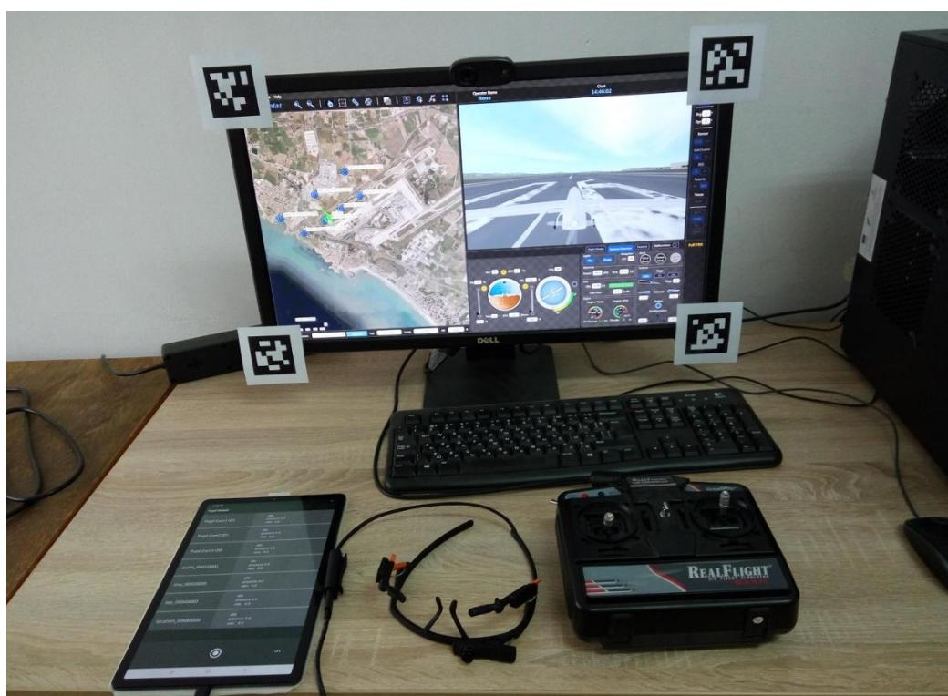
Fig. 1. C-Star simulator (SimLat, Inc.): pilot station equipped with Pupil Labs Core eye tracker
