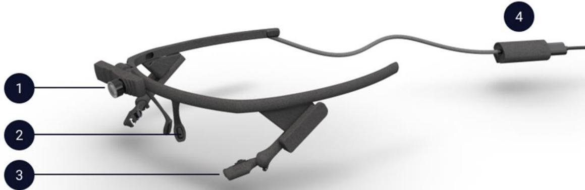
**Fig. 2. Pupil Labs Core binocular headset:** 1) World camera; 2) Nose clip; 3) NIR camera and IR LED @ 850 nm; 4) USB-C connector
