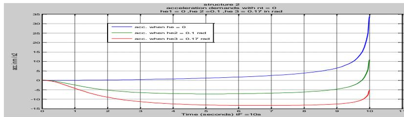
Figure 18: Acceleration demands( $m/s^2$ ),  $nt = 0$ , deferent Head errors, structure 2
