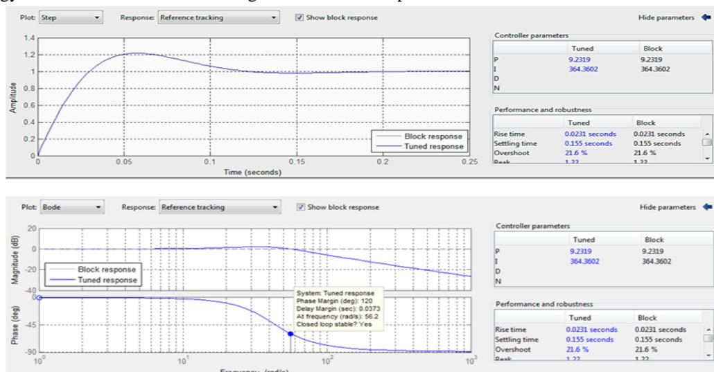
Figure 42: Time and Frequency domain of PI parameters used to improve structure
