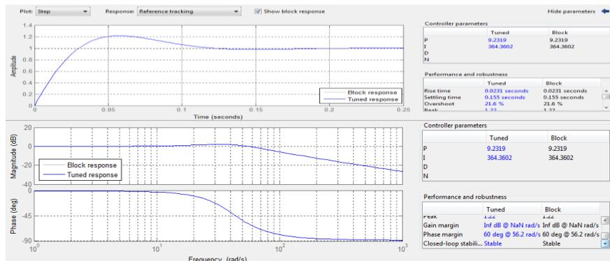
Figure 23: Time and Frequency response of PI controller of structure 1
