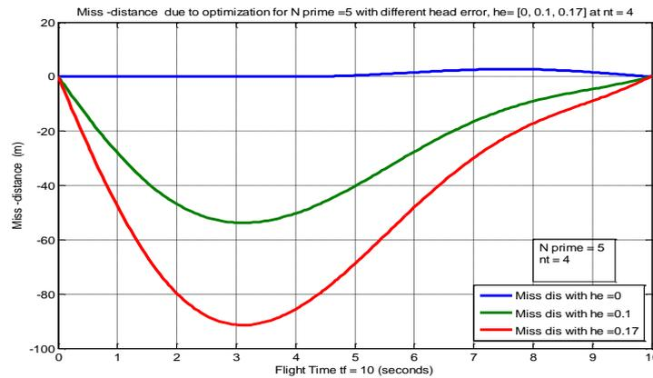
Figure 37: Optimal miss distances  $n_t = 4$ ,  $N_{prime} = 5$ , with different head errors.
