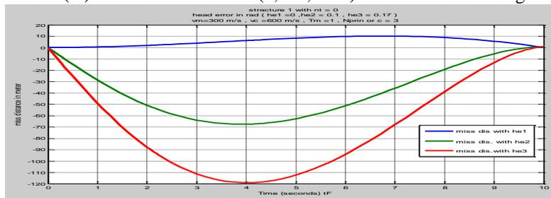
Figure 9: Miss distance (m),  $nt = 0$ , different Head errors, structure 1
