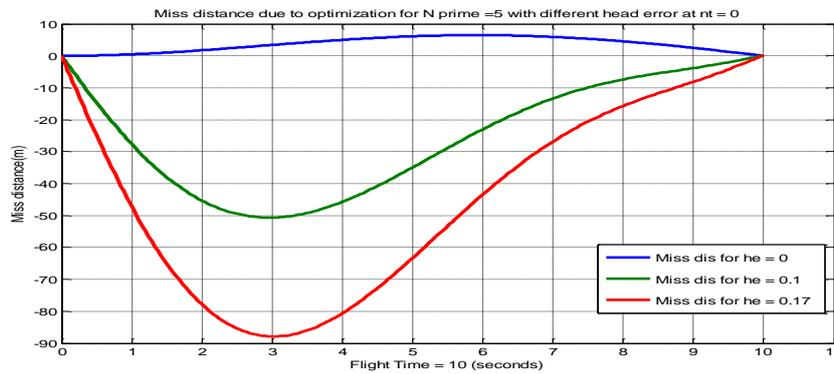
Figure 35: Optimal miss distances  $nt = 0, N \text{ prime} = 5$ , with different head errors
