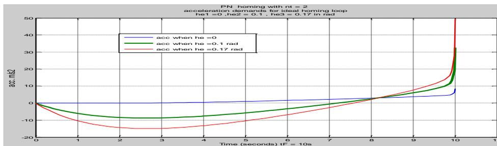
Figure 4: Acc. demands( $m/s^2$ ),  $nt = 2$ . He (0, 0.1, 0.17) of Ideal homing loop. Table(2) shows the comparing between main parameters, when the target acceleration ( $nt = 2$ ) and head error has ( $He_1 = 0$ ,  $He_2 = 0.1$  rad,  $He_3 = 0.17$  rad ).
