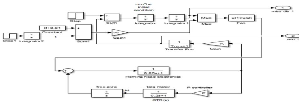
Figure 15: Block diagram of PN homing with free gyro. Structure 2
