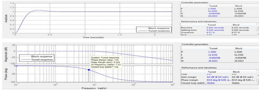
Figure 24 :Time and frequency domain of PID parameters and different values N'
