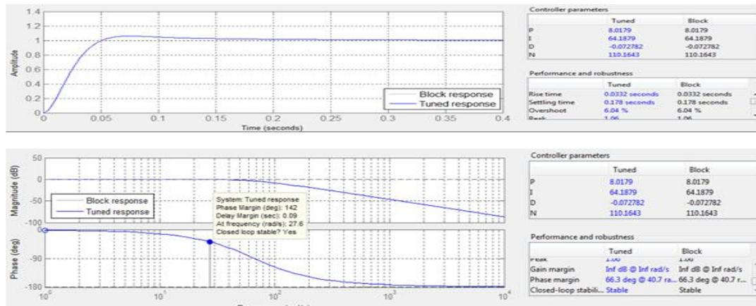
Figure 34: Time and frequency response of PID used for N prime = 5, used for improvement.
