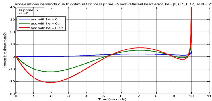
Figure 39: Optimal Acc. demands,  $nt = 2, N \text{ prime} = 5$ , with different head errors
