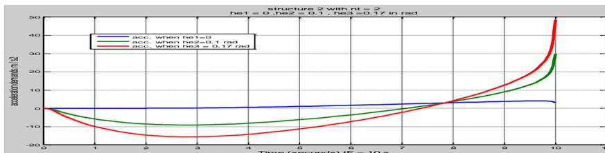
Figure 20: Acceleration demands( $m/s^2$ ),  $nt = 2$ , deferent Head errors, structure 2.
