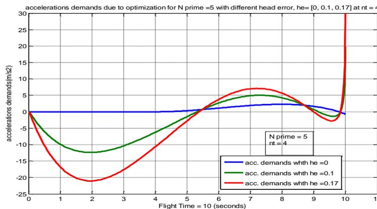
Figure 41: Optimal Acc. demands,  $n_t = 4$ ,  $N_{prime} = 5$ , with different head errors
