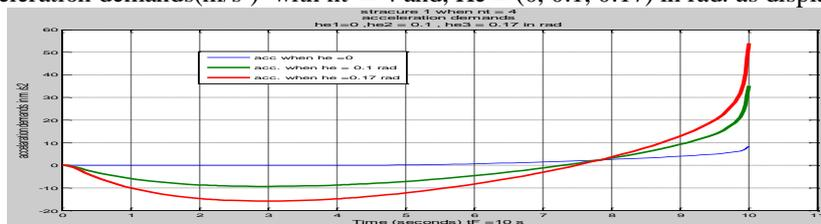
Figure 14: Acceleration demands ( $m/s^2$ ),  $nt = 4$ . deferent Head errors, structure 1
