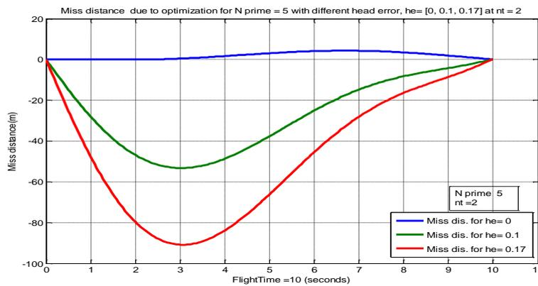
Figure 36: Optimal miss distances  $nt = 2, N \text{ prime} = 5$ , with different head errors
