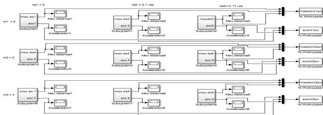
Figure2: Full Simulink diagram of proportional navigation an ideal homing loop
