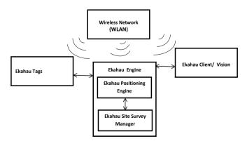
Figure 3.1: The Block Diagram of Ekahau RTLS System [19]
