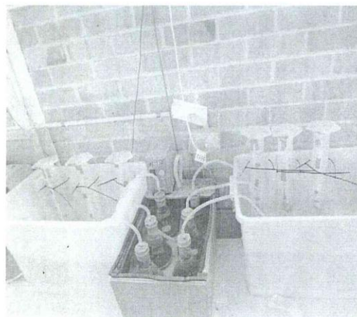
Figure 14: A Batch Type Anaerobic Digester Producing Biogas (picture gotten from the lab)
