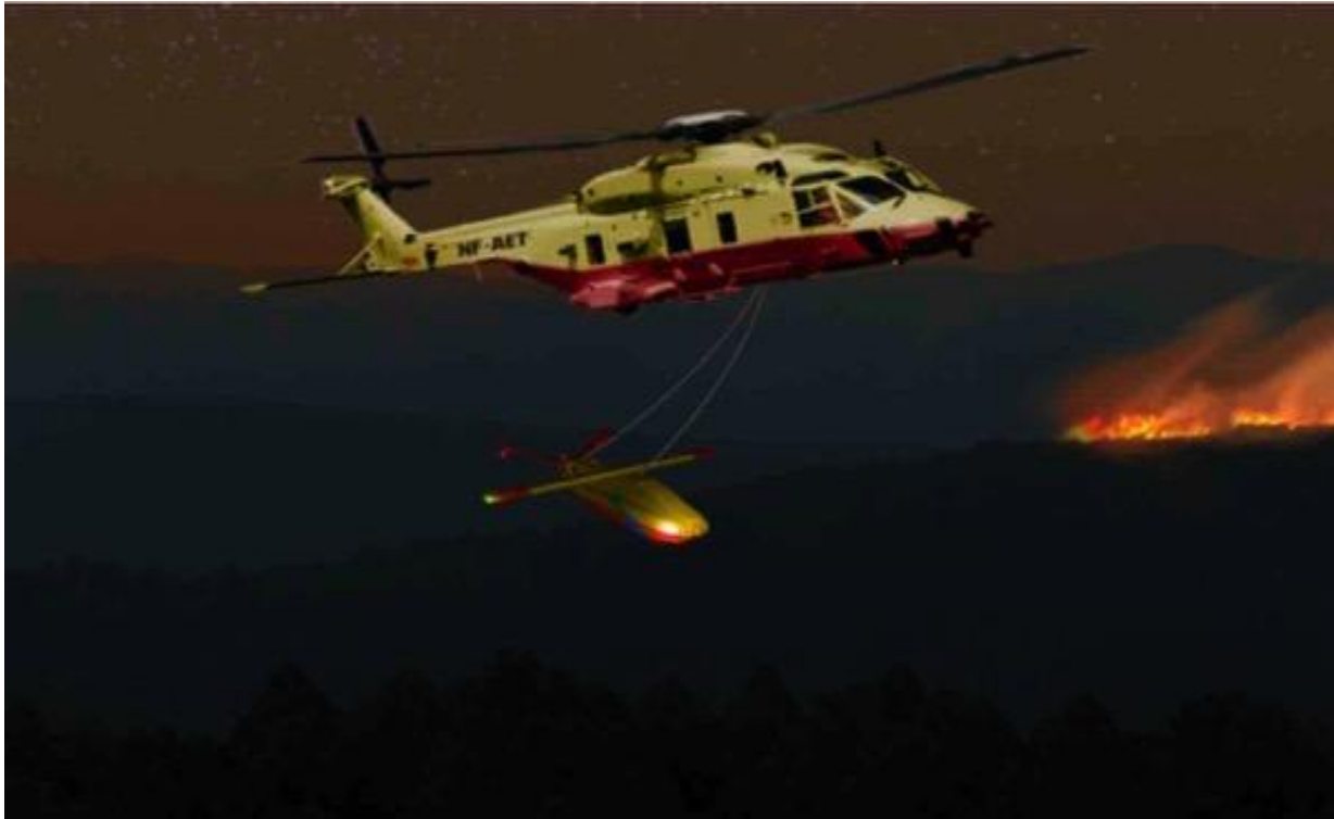
Fig. 17: Launching of AGCs from the LA (heavy/medium cargo helicopter) at night
