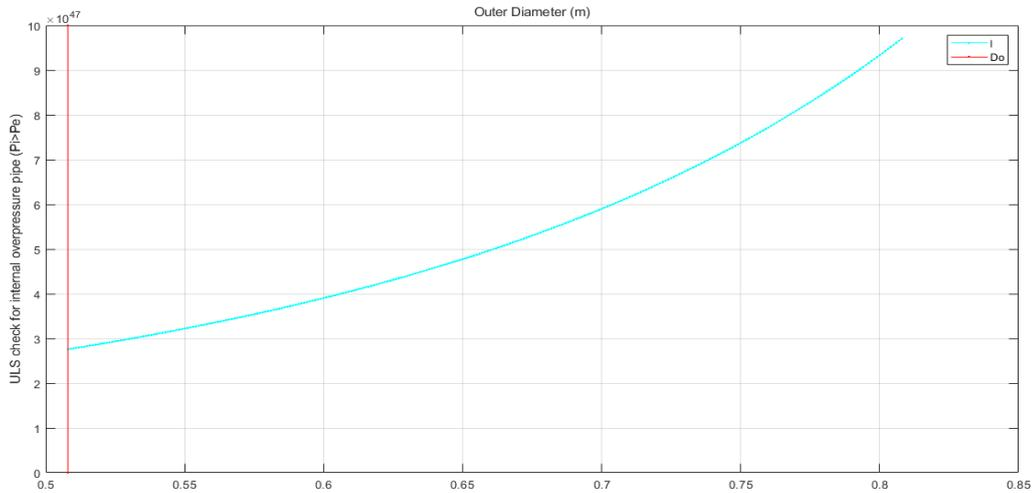
Figure 8: Outer diameter vs ULS check for internal overpressure pipe ( $P_i > P_e$ )
