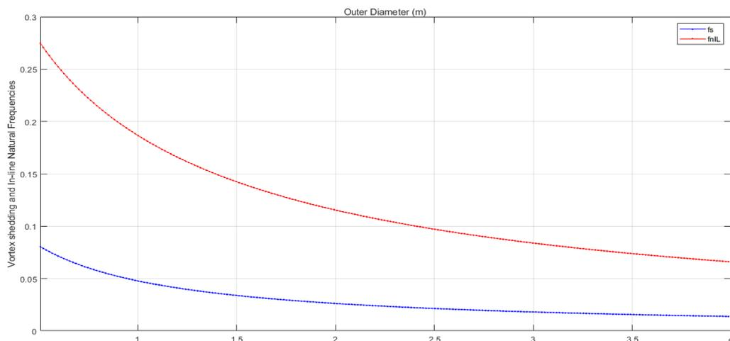
Figure 9: Outer diameter vs Vortex shedding frequency and In-line Natural frequency
