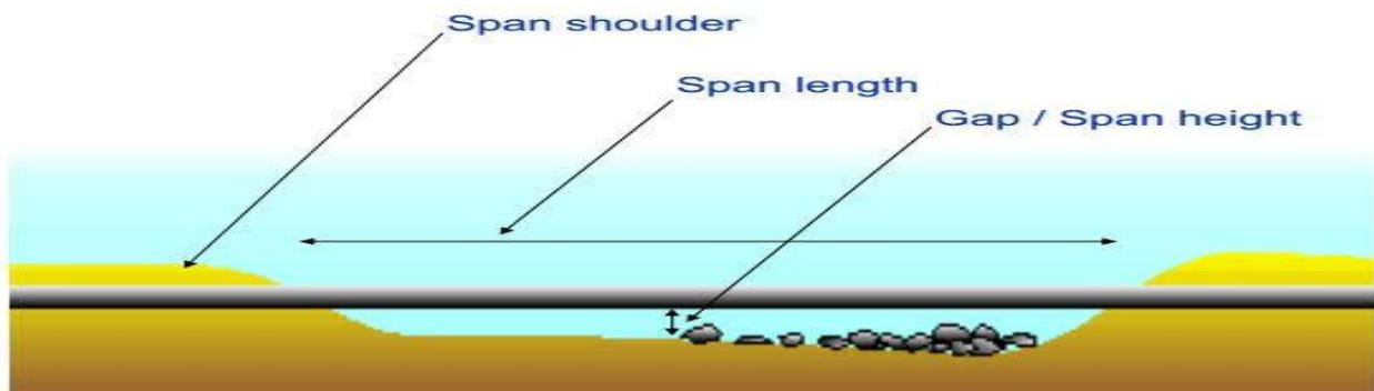
Figure 1: Free spanning section of an offshore pipeline [2]
