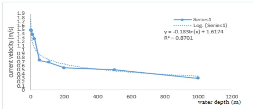
Figure 5: Current Velocity Profile
