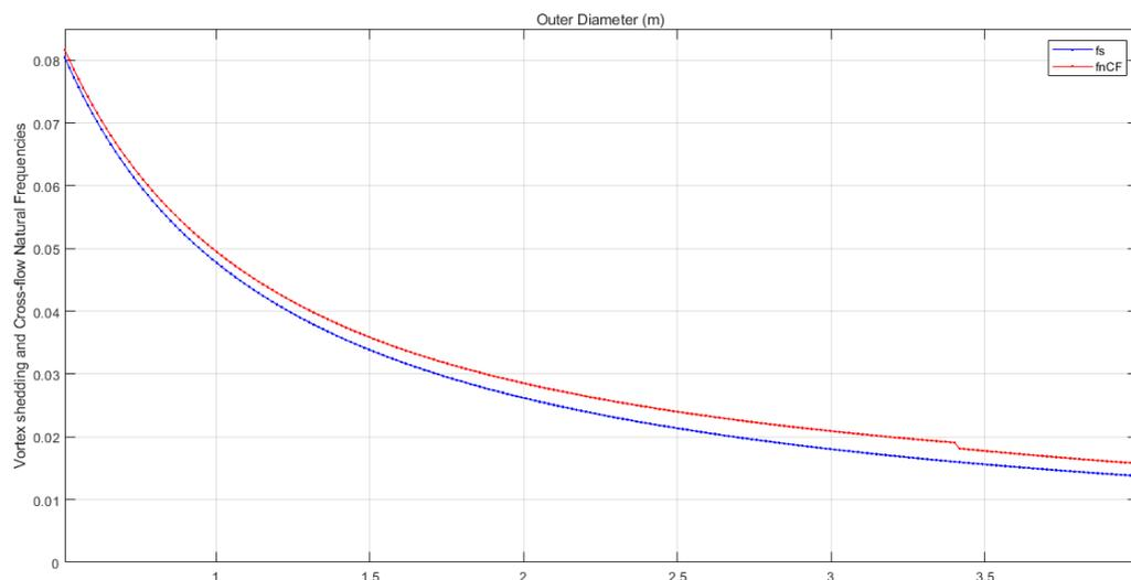
Figure 10: Outer diameter vs Vortex shedding frequency and Cross-flow Natural frequency
