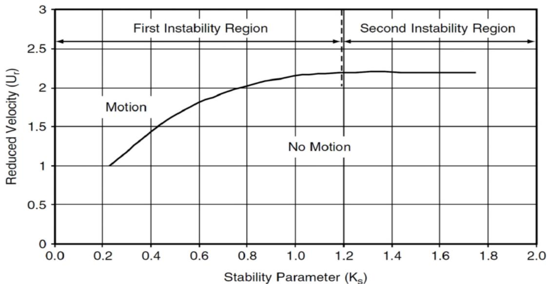
Figure 3: Relationship between Reduced Velocity and Stability parameter.
