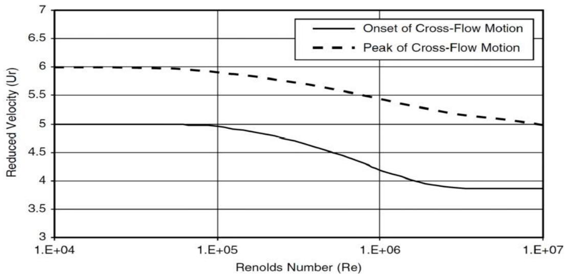
Figure 4: Relationship between Reduced Velocity and Reynolds Number
