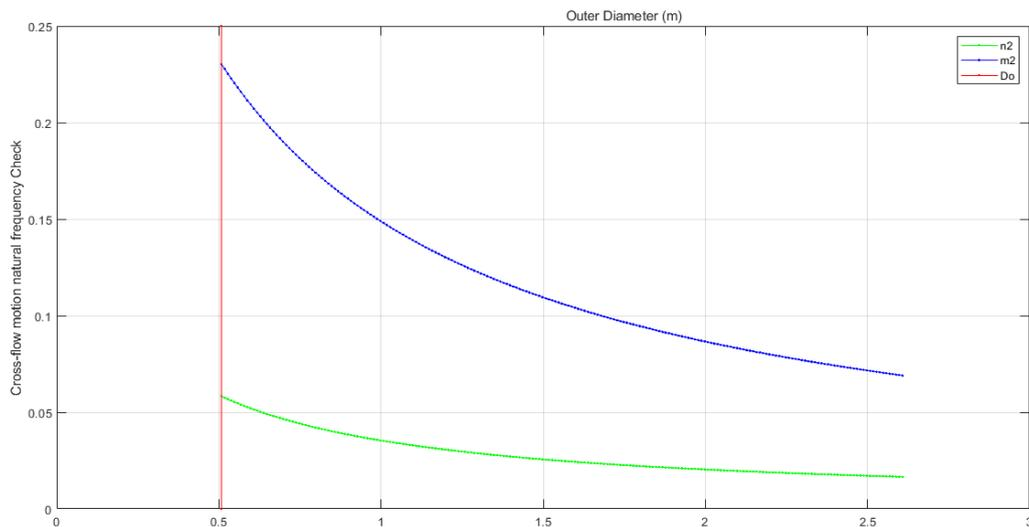
Figure 7: Outer diameter vs Left and Right-hand side of Cross-Line motion natural frequency check
