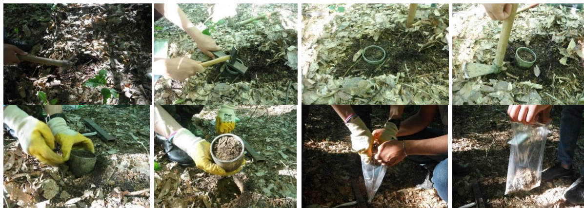
Figure 4. Soil samples taken from the upper soil level (Varol et al., 2020)
