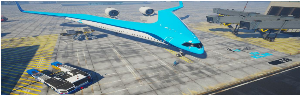
Figure 5. Flying-V aircraft concept developed by TU Delft in collaboration with KLM
