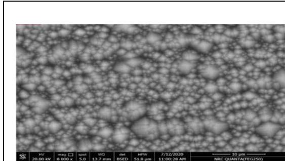
**Fig.7.SEM images of silicon surface after etching at (0.3357 mol) KOH concentration.**
