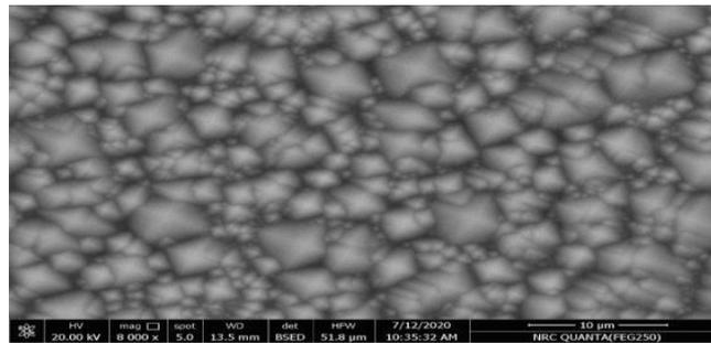
**Fig.11. SEM pictures of mono crystalline silicon surface after etching for (20 minutes) time period.**
