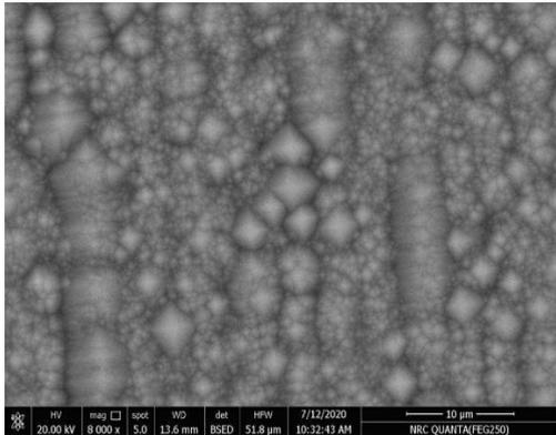
**Fig.9. SEM pictures of mono crystalline silicon surface after etching for (7 minutes) time period.**
