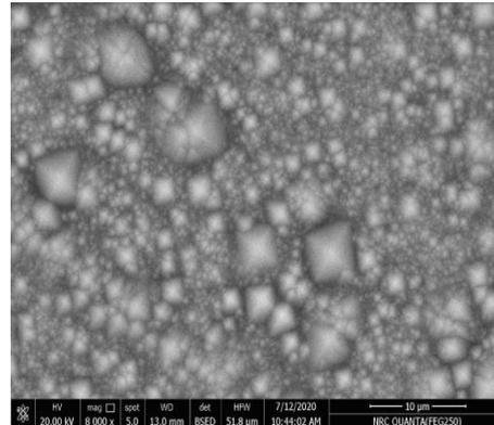
**Fig.10. SEM pictures of mono crystalline silicon surface after etching for (14 minutes) time period.**
