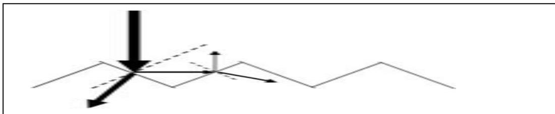
Fig.2. showing an increase in the path of the photon falling on the surface of the cell, after the texturing process .
