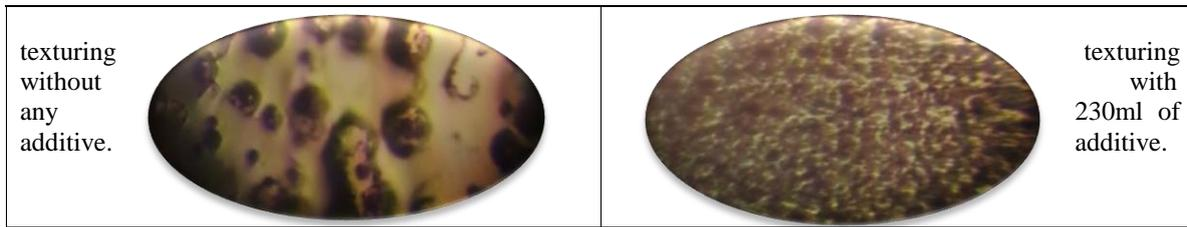
in the case of the addition of an active material less than 230 ml affect the homogeneity of the surface of the cell as it pyramids are not homogeneous on the surface in addition to the emergence of some Spots resulting in the addition of the active substance by 230 ml in the potassium hydroxide solution basin in the Egyptian National Laboratory for Renewable Energy to obtain a homogeneous and shiny surface free of spots.
