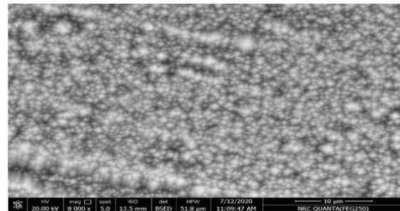
**Fig.8.SEM images of silicon surface after etching at (0.1678 mol) KOH concentration.**
