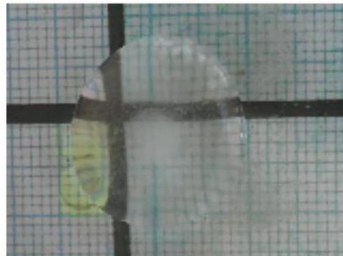
(d) Continuous surface waves: overlapping between the surface disturbances and the propagating air wave.
