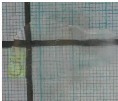
(i) Finally, the drop is fully dislodged under the drag force pushing the liquid molecules downstream the air jet.
