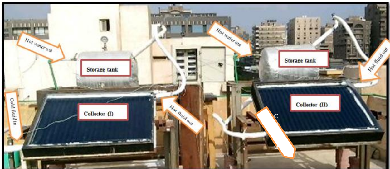
Fig. 2: A homemade of flat-plate solar collectors equipped with water tank for the first experiment.
