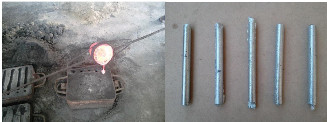
Figure 2 (a) Pouring Molten Metal into the Mold (b) Cast A356.2/FA Composites
