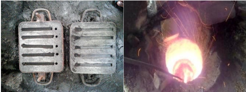
Figure 1 (a) Preparation of Mold (b) Mixing A356.2 and Fly Ash
