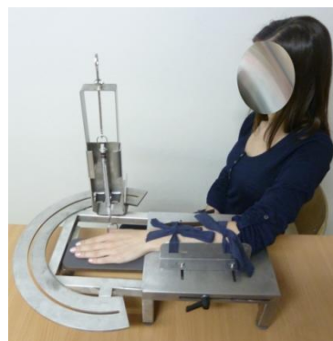
Figure 7: Measurement Process Using a Spring Dynamometer.
