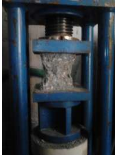
Figure 3. Compression Failure of cube
