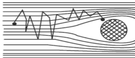
Figure 3: Brownian diffusion - The particles traverse the flow stream, they collide with the fibre and are collected.
