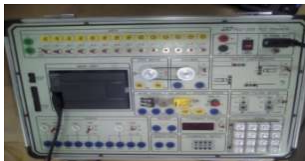
Figure 1: PLC trainer (SIEMENS SIMATIC S7-200 PLC inside)
