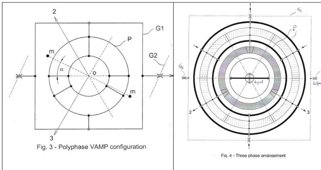
The resultant AM arbitrarily positioned in the plane P can be treated as a composite gyro having similar properties as the dual DC motor model [1]. That means if any torque applied to the platform P the system will react as per well-known gyro properties. The said torque can be arbitrarily positioned in the space having two components i.e. in the plane P and perpendicular over it. Both components will generate adequate reaction of the AM.
