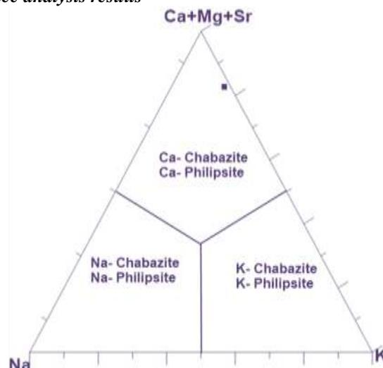
**Fig. 5:** Classification plot for zeolite (after Weisenberger and Spurgin, 2009). Sample classified under Chabazite, depleted in Na, and plot closer to Ca+ Mg + Sr. thus less enriched in K.
