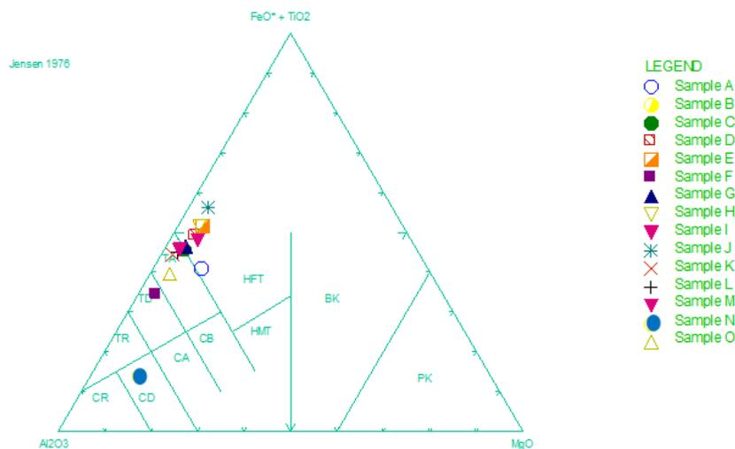
Fig. 4: AFM Ternary (cation percent; Jensen, 1976) plot for Tim-kwalla basalts. HFT – High Fe tholeiite; HMT = High Mg tholeiite; BK basaltic komatite; PK = peridotitic komatite; T = tholeiite; C = calc-alkaline, B = basalt, D = dacite, R = rhyolite).
