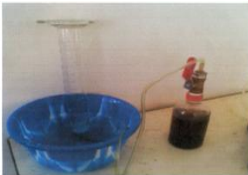
Fig 2: Measurement of the biogas using water displacement method.
