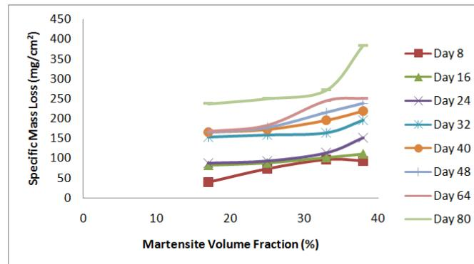
Fig. 8: Specific Mass Loss versus Martensite Volume Fraction
