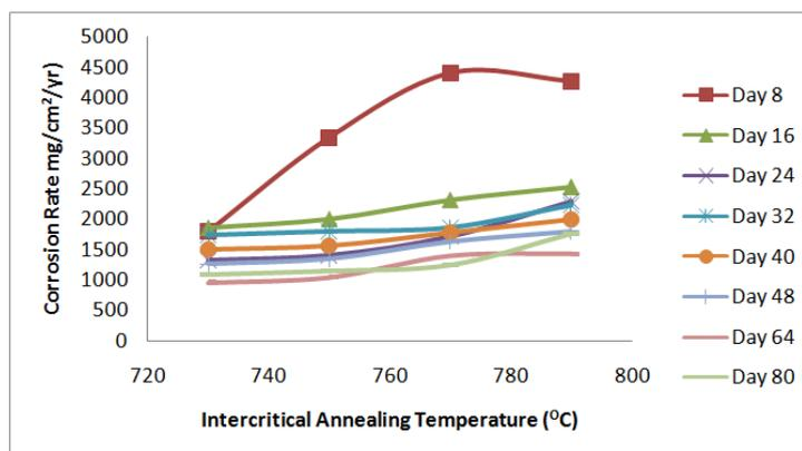
Fig. 7: Corrosion Rate versus Intercritical Annealing Temperature
