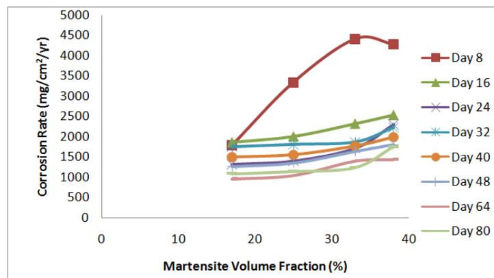
Fig. 9: Corrosion Rate versus Martensite Volume Fraction
