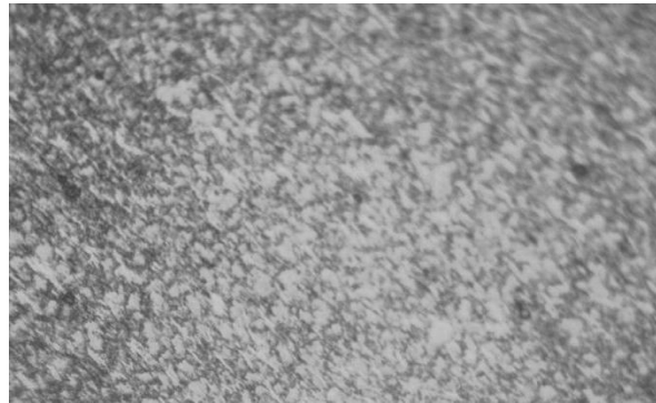
Fig. 2: Photomicrograph of Normalized sample
