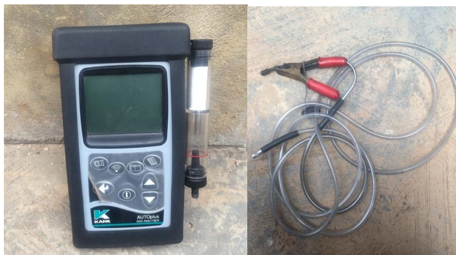
(i) Exhaust Gas analyzer (ii) Exhaust gas probe of the gas analyzer
