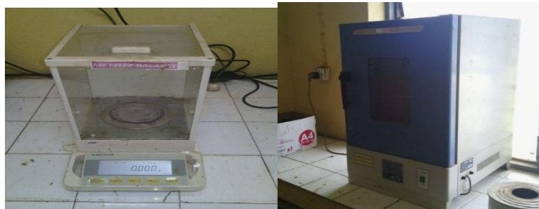
(i) Mettle balance for weighing samples. (ii) Oven used for drying samples.
