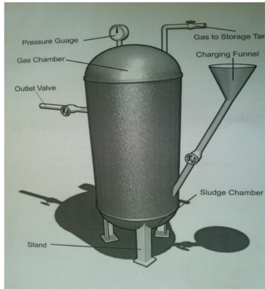
Plate 1: Fabricated Anaerobic Digester
