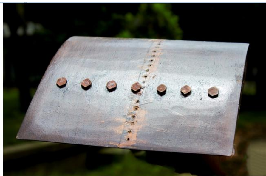
Fig. 2(b). Constructed model with hexagonal dimples
