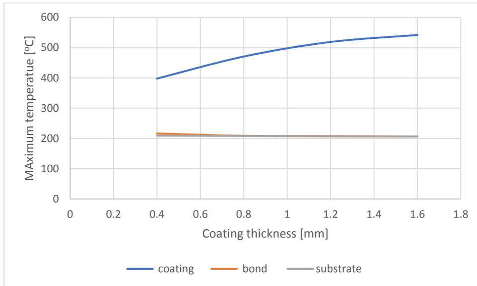
Fig 6: Maximum temperature distribution as a function of coating thickness.
