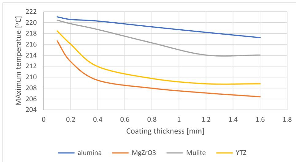
**Fig 8:** Maximum temp distribution at substrate surface as function of coating material.
