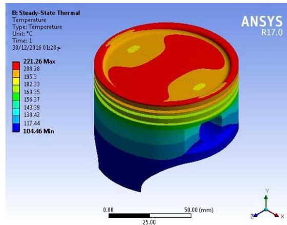
Fig 3: Temperature (°C) contours on the uncoated piston SI engine.
