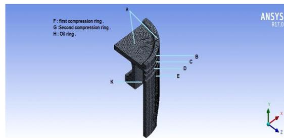
**Fig 2:** The meshing of piston and the thermal boundary condition of the piston used in the FE Analysis.
