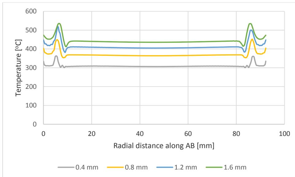
**Fig 5:** Top surface temperature distribution with coating along the radial distance.
