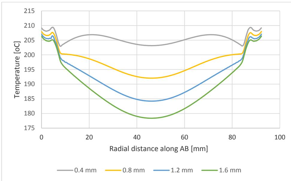
**Fig 4:** Substrate surface temperature distribution with coating along the radial distance.
