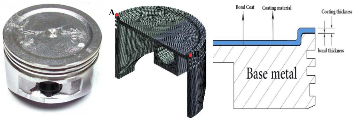
**Fig 1 :** The model used in the FE analyses: photograph of the partially coated piston, and the half part of the model and the parameters.
