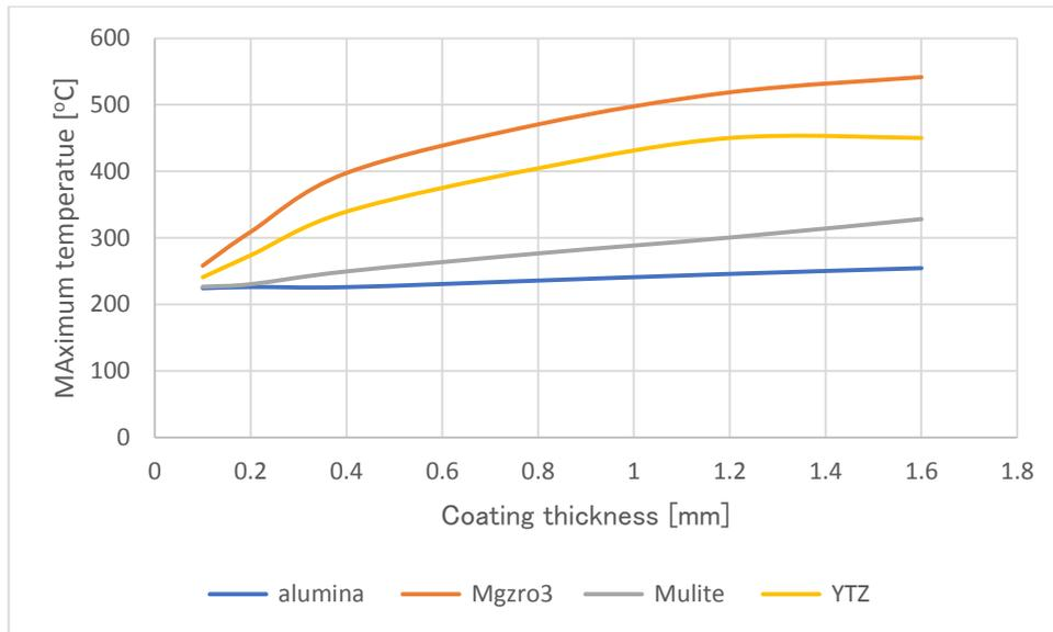
**Fig7:** Maximum temp distribution at top coating surface as function of coating material.
