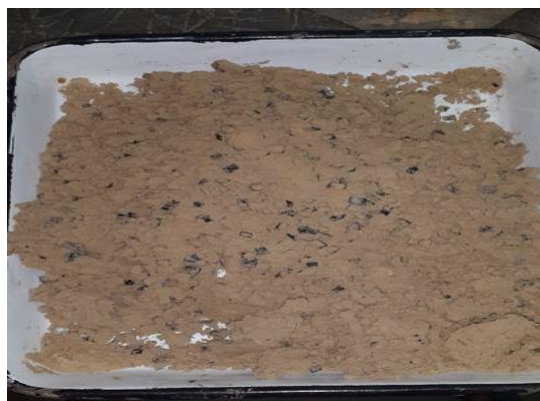
Figure 1: Plastic Waste Strips Mixed with Dune Sand
