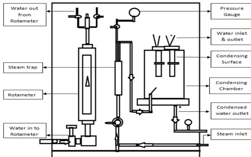
**Figure 2:** Schematic Diagram of Dropwise Condensation Apparatus
