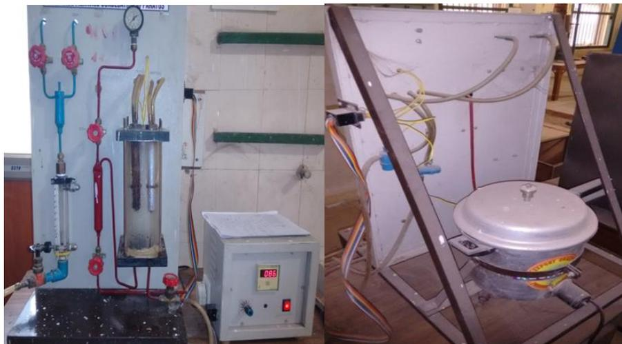
**Figure 3:** Front View and Back View of Dropwise Condensation Apparatus
