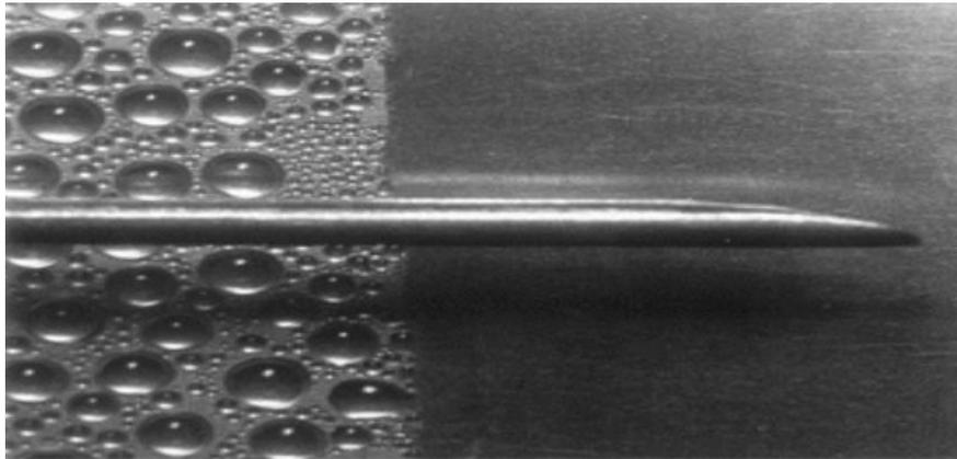
**Figure 1:** Dropwise & Filmwise Condensation on Vertical Surface [2]
