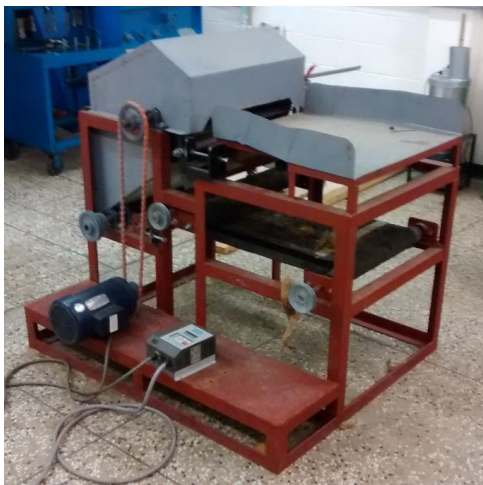
Figure 1. Slotted-barrel rotating machine used to extract the banana fibre
