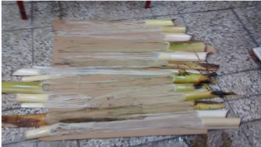
Figure 3. Processed banana strips showing exposed fiber
